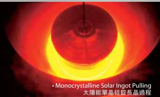
• Monocrystalline Solar Ingot Pulling
