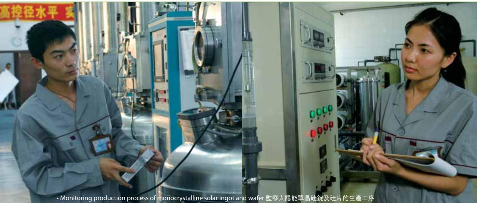
• Monitoring production process of monocrystalline solar ingot and wafer 監察太陽能單晶硅錠及硅片的生產工序
